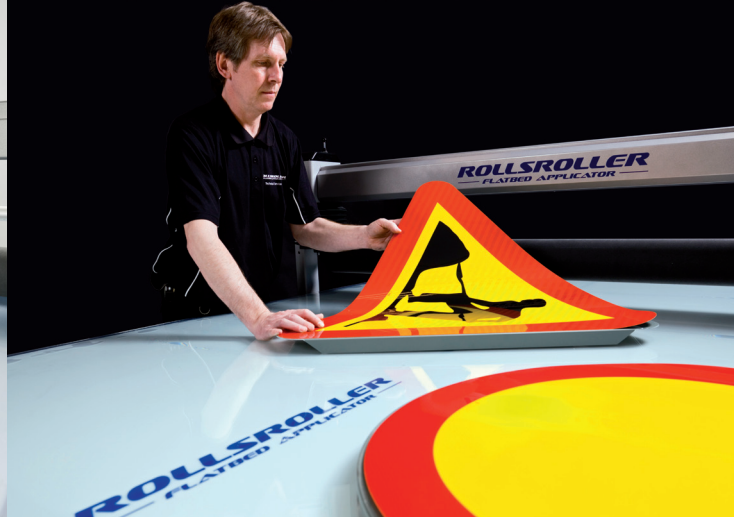
Easy mounting of pre-masking tape onto electronic cuttable overlay film (ECOF).
